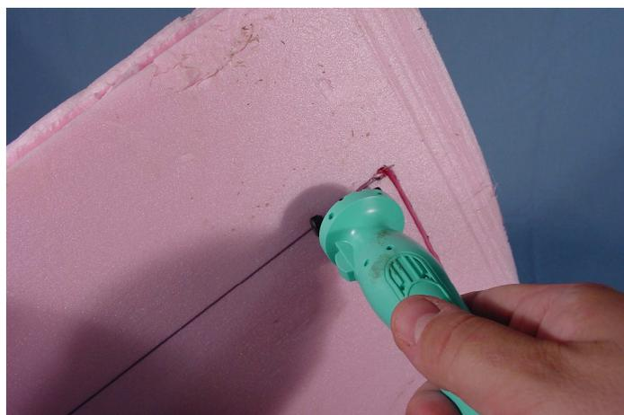
*Once you have laid out the scene on a large sheet of foam you can use a hot knife to cut out the base.*
